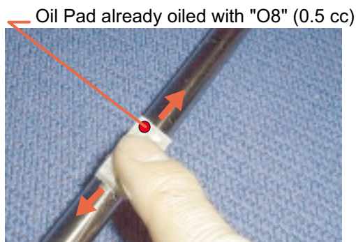
Figure 6-6. Preliminary Lubrication with "O8"
